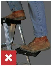
DON'T stand above the second step from the top of a stepladder or the fourth rung from the top of an extension ladder. DON'T climb on the back of a stepladder. DON'T stand or sit on a stepladder top or pail shelf.
