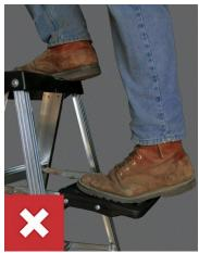
DON'T stand above the second step from the top of a stepladder or the fourth rung from the top of an extension ladder. DON'T climb on the back of a stepladder. DON'T stand or sit on a stepladder top or bucket shelf.
