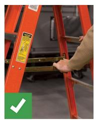
Properly set up and use the ladder in accordance with safety instructions and warnings. Wear shoes with non-slip soles. Center body on the ladder and keep belt buckle between the rails while maintaining a firm grip. OSHA has a Quick Card available on ladder safety. This could be a topic for a tailgate safety meeting. <a href="https://www.osha.gov/sites/default/files/publications/portable\_ladder\_gc.pdf">https://www.osha.gov/sites/default/files/publications/portable\_ladder\_gc.pdf</a>
